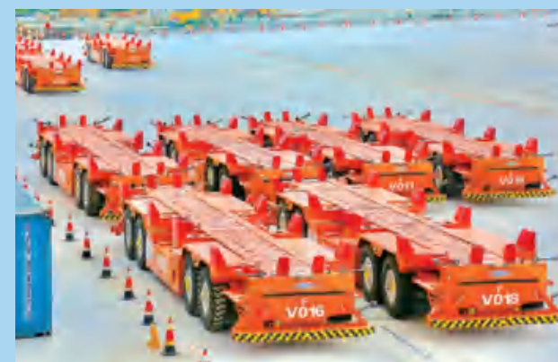
The world's first unmanned intelligent IGV navigated by Beidou
