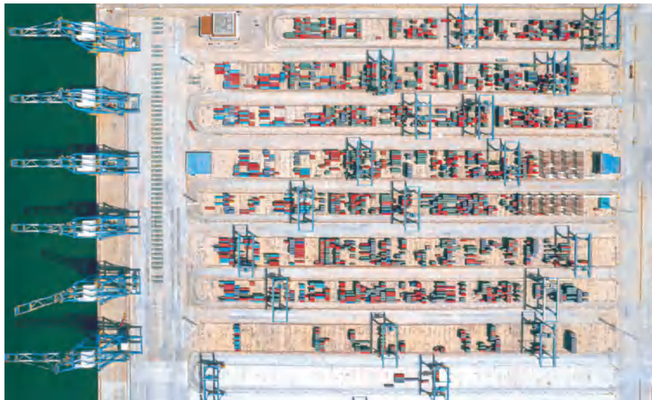
The Qinzhou automated terminal with the U-shaped process layout at Beibu Gulf Port
